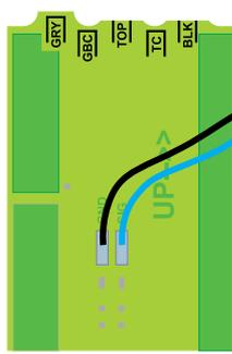
Example of corrected FRESH TOP sender programming (GRY or BLK tab cut by mistake)
