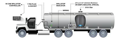
The SpillStop consists of three main components: the controller in the cab of the truck, the optional plug module inside the 7 pin socket housing on the trailer, and the gauge module inside the SeeLeveL truck gauge (the gauge module is built into the 808P2 and 810PS2 displays).
