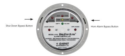
The 815U alarm controller monitors and displays the alarm status of the gauge, and activates a horn if the fluid level in the truck tank is at the full point, and shuts off the pump or vehicle engine if a spill is imminent. Each 815 Ultra controller accommodates one compartment. **WARNING:** The SPILLSTOP ULTRA is intended as an emergency backup system only, and is not intended as a substitute for operator diligence during the loading process.
