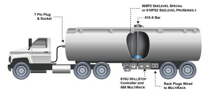
The SPILLSTOP consists of three main components: the controller on the truck, the optional plug module inside the 7 pin socket housing on the trailer, and the gauge module inside the SeeLeveL PROSERIES truck gauge (the gauge module is built in to the SeeLeveL Special display).
