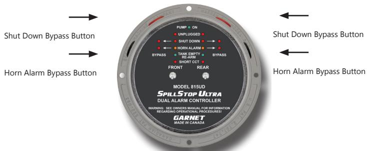
The 815UD alarm controller monitors and displays the alarm status of the gauges, and activates a horn if the fluid level in either truck tank is at the full point, and shuts off the pump if a spill is imminent. The 815UD controller accommodates two compartments.
