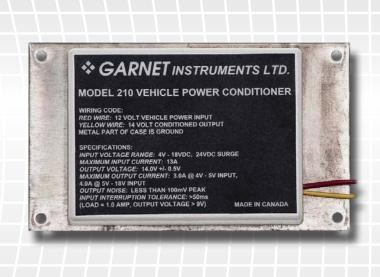
The Garnet Model 210 Vehicle Power Conditioner maintains a constant 14V output despite variations in voltage from the vehicle's electrical system. It permits proper equipment operation despite inadequate electrical system voltage, and protects equipment from voltage surges of either polarity. Ideal for operating voltage-sensitive equipment such as sensors, computers, and communications systems.
