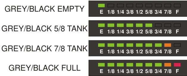
2. If no other button is pressed, then the display will shut itself off after about 5 seconds. If the button is held down, the display will recheck the level once per second and will show the updated level.
