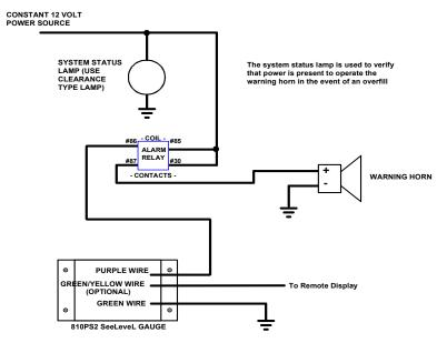
A relay is needed when the warning device draws greater than 1 amp.
