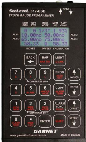
The **SEELEVEL™** 817-USB Truck Gauge Programmer is used to program tank calibrations and alarms and to troubleshoot any **SEELEVEL™** 800 series systems. The USB interface allows tank calibration files to be created and stored on a PC computer.
