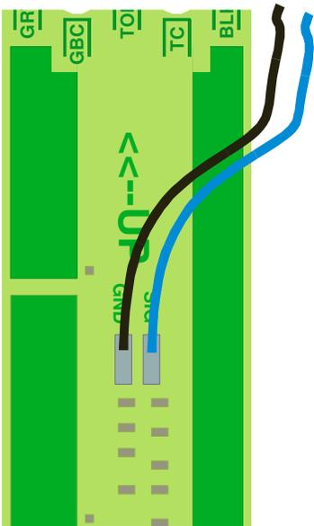
Example of corrected GREY SINGLE or BOTTOM sender programming (BLK cut by mistake)
