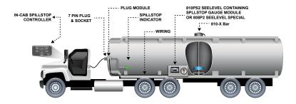
The SpillStop consists of three main components: the controller in the cab of the truck, the optional plug module inside the 7 pin socket housing on the trailer, and the gauge module inside the SeeLeveL truck gauge (the gauge module is built into the 808P2 and 810PS2 displays).
