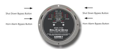
The 815UD alarm controller monitors and displays the alarm status of the gauges, and activates a horn if the fluid level in either truck tank is at the full point, and shuts off the pump if a spill is imminent. The 815UD controller accommodates two compartments.
