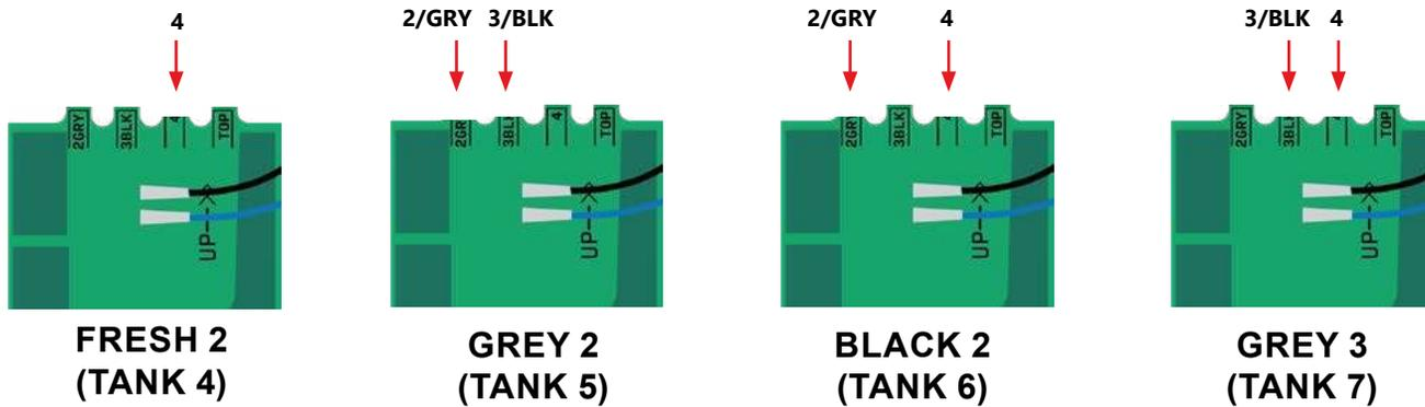
**CAUTION:** MAKE SURE YOU CUT THE CORRECT TABS! Cutting the wrong tabs will result in incorrect programming and this cannot be reversed and is not covered under warranty
