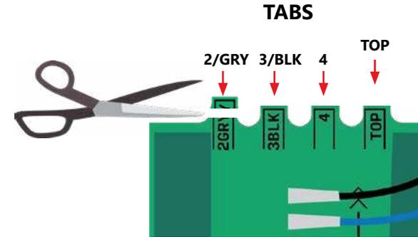
Senders are programmed by cutting off the tabs at the top of each sender to tell it which tank it will be mounted on, or if in a stacked configuration, whether they are on the top or bottom. A pair of scissors or a hole punch can be used to cut the sender tabs.
