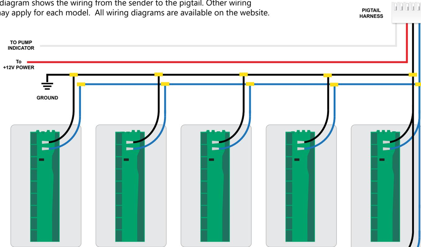
Up to 7 tanks can be connected.
