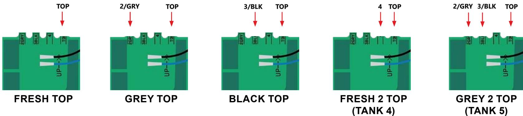
For Tanks 4 - 7 also cut the TOP tab as these examples indicate.
