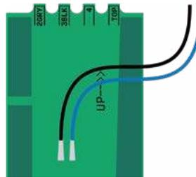
Wires from 710-ES2 sender have a vertical orientation
