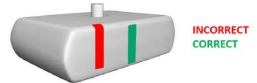
**CAUTION:** Bending the sender sharply will damage the circuit on the sender.
