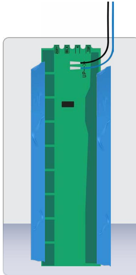
**⚠ CAUTION:** Route wires to the right, away from the senders. The wires indicate the top of the sender.
