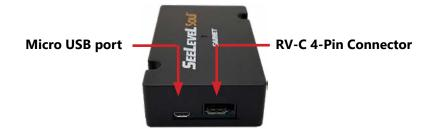
**Micro USB port:** Used to connect the module to a computer for configuration purposes. A standard Micro-USB cable can be used. **RV-C CAN Connector:** provides an extra CAN BUS connection.
