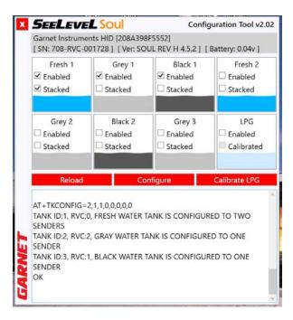
7. The "**Reload**" button on the configuration tool is used to simulate a disconnection from the unit being configured and trigger a full reload of the working settings (Soul -> PC).
