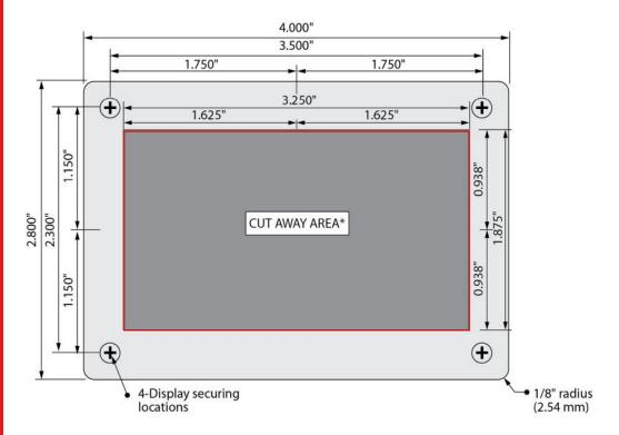
**CAUTION:** If mounting the display in a metal panel or wall there is a risk the display can short circuit causing permanent damage. Non-conductive mounting spacers are available to purchase to help prevent damaging the display. Contact Garnet or go to our website for further details. More installation tips are available in the "Troubleshooting and Installation Tips" section.
