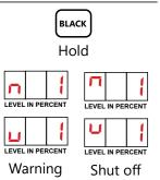
A NOTE: All alarms are tied to the single common alarm output. Additional alarms are possible with the external alarm module.
