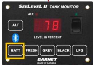
Press BATT button to enable search mode for 10 seconds.
