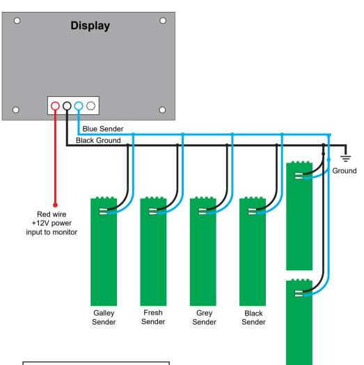
A WARNING: All power circuits must be fused. If a fuse is not provided with the system then it is the installer's responsibility to install a fuse with the maximum rating your model requires.
