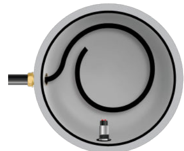
Figure 3.4.2a Fiber Optic Cable in Enclosure
