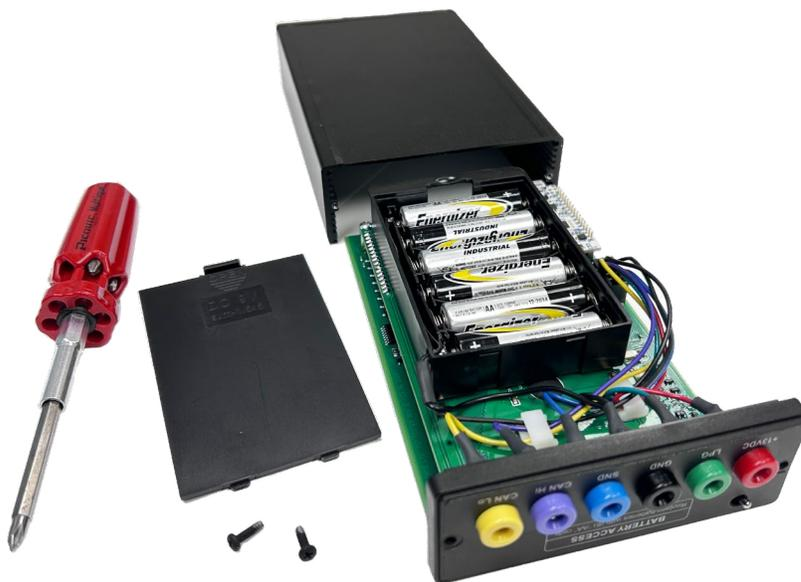
**Figure 2.4a** Replacing Batteries
