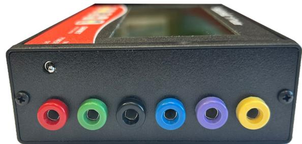
Figure 2.3a 717 Tester Connectors
