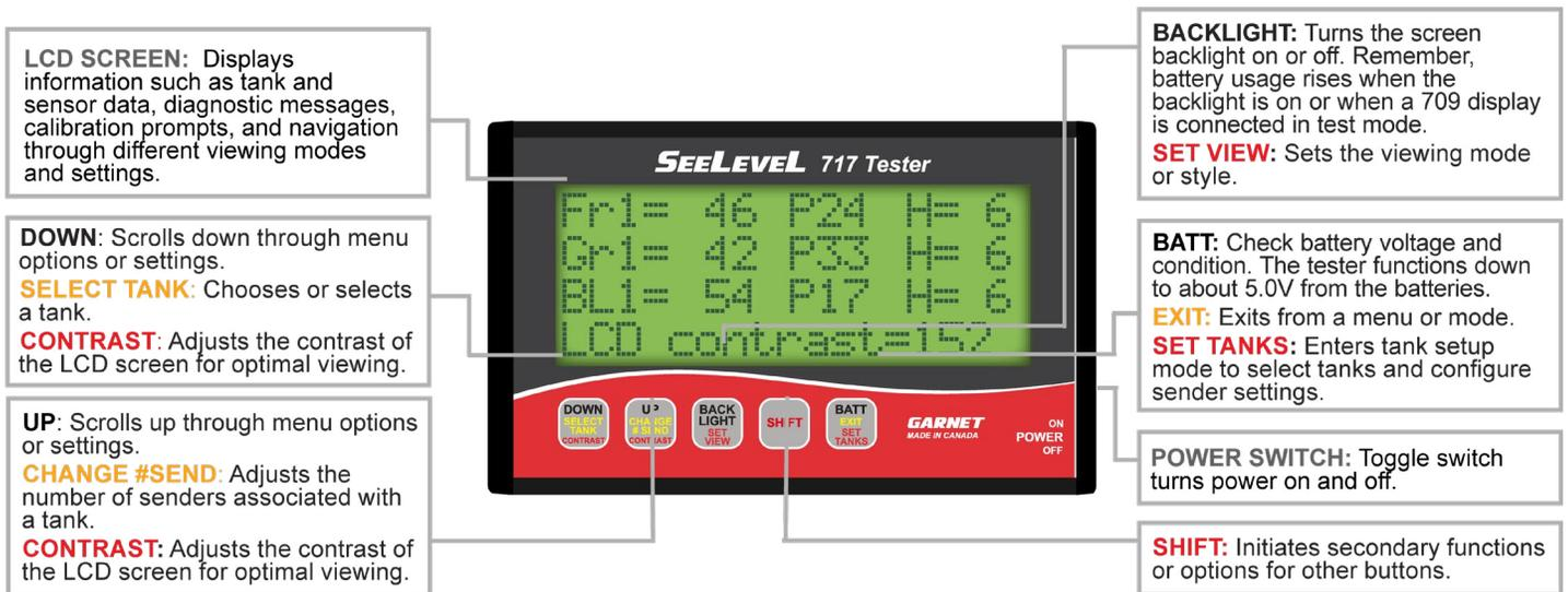
Figure 2.2a Front Panel Display
