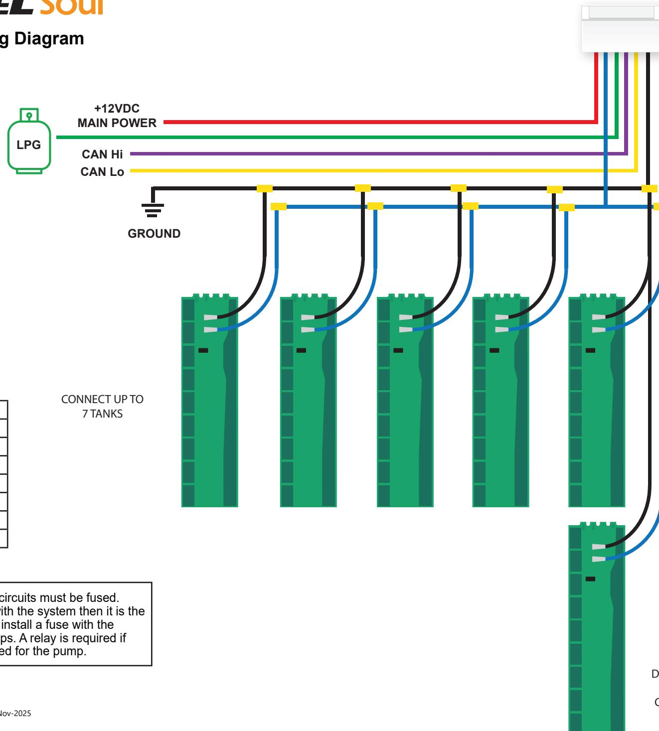
**WARNING:** All power circuits must be fused. If a fuse is not provided with the system then it is the installer's responsibility to install a fuse with the maximum rating of 7.5 amps. A relay is required if more than 7.5 amps needed for the pump.
