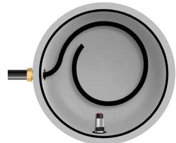
Figure 3.4.2a Fiber Optic Cable in Enclosure
