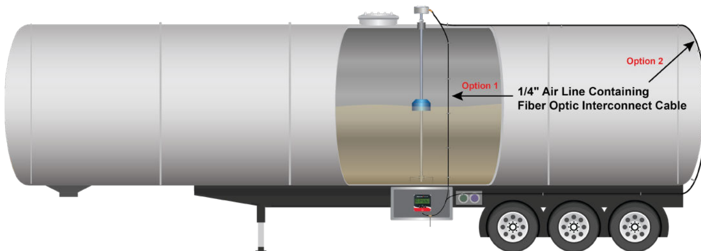
Figure 3.r Air Line Routed from Sender Bar to Gauge
