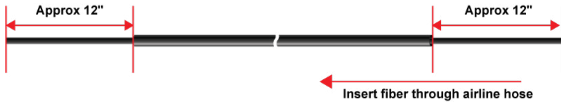
Figure 3.m Fiber Optic Cable Inserted Through Air Line Hose
